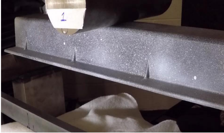
Test run 1 – elevated elongation, lower yield strength and UTS. Higher displacement and energy absorption
